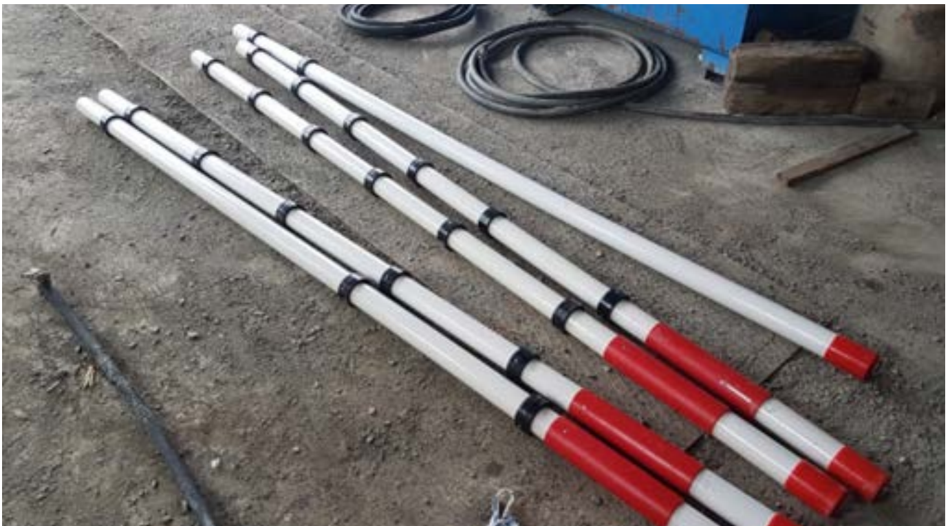
Inclinometer -Magnet-Extensometer borehole casing prepared to have the temperature strings attached: ready to install
