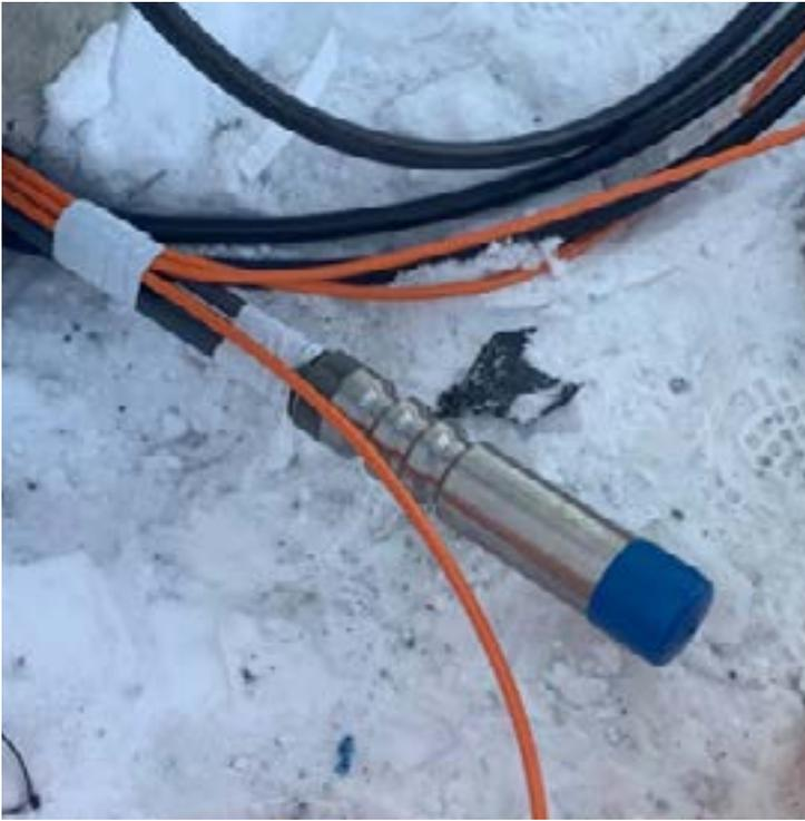
Borehole extensometer head (type Huggenberger) with cables of temperature string
