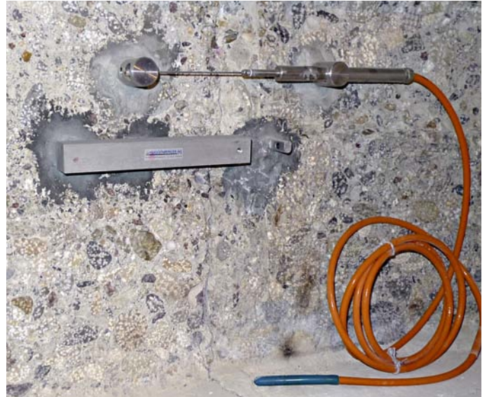
TJM1DS type for the 1-dimensional surveillance of joints and cracks
