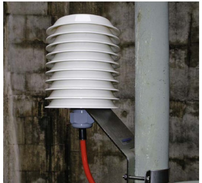
TA type with Shelter (weather and radiation protection)
