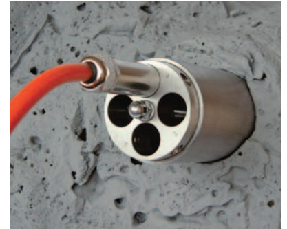
RM T4; 4 rods with electrical transducers for automatic measurement
