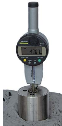
RM3; 3 rods with Setdeflectometer for manual measurement
