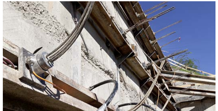
Load cell PRE 1000/100/80 monitoring a retaining wall
